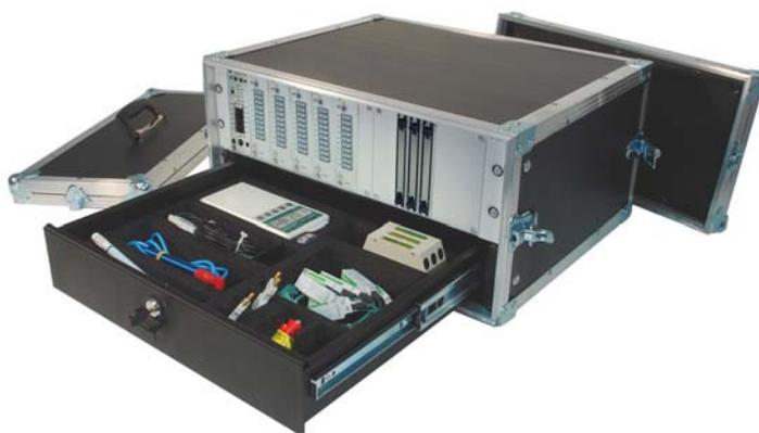
Rack case with carrying handle, for ALMEMO® MA5690xxBT8 measuring systems, in 19-inch sub-rack
